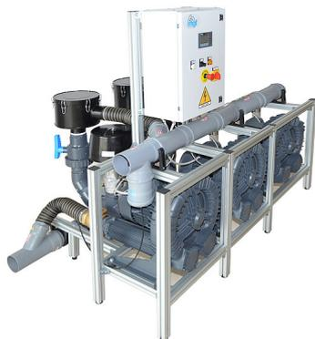
Centralized dry suction system for 45-60 units in simultaneous operation, consisting of 3 ASPIR 8 16.5 kW suction units. control unit with PLC for automatic activation of vacuum threshold pumps, complete with pressure sensor, regulation, alarms, inverter. Total three-phase power output at 50 Hz, 16.5 kW 400V, maximum flow rate of 18,000 l /min, at a maximum operating head for continuous service of 160 mbar. Complete system of 3 HEPA antibacterial filters.
