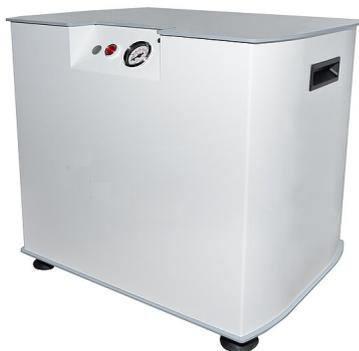
Super silent twin cylinder oil free compressor, dB 50/1m, 1400 rpm, maximum pressure 7 bar, 3 liter stainless steel tank and is available in both stationary and wheeled versions (code with - C at the end).
