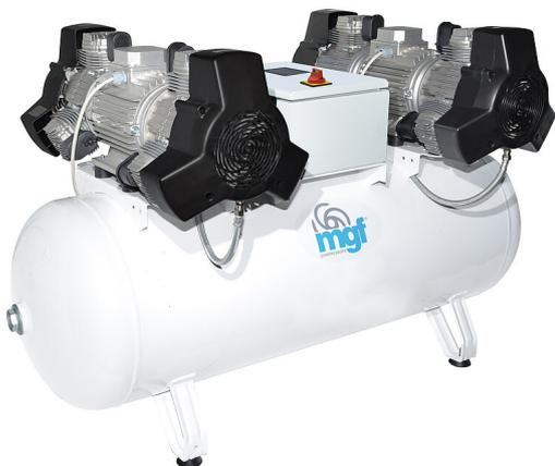
Three-phase dry air compressor IOT version, 12 cylinders, with an air output of 900 l/min at 5 bar pressure. Tank capacity 270 L, internal surface treatment to protect against corrosion.
