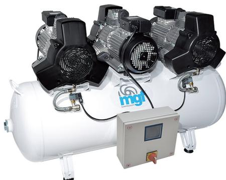
Three-phase dry air compressor IOT version, 9 cylinders, with an air output of 750 l/min at 5 bar pressure. 200 L tank capacity, internal surface treatment to protect against corrosion.
