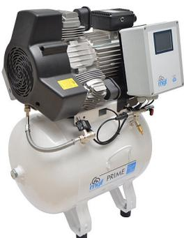
IOT version oil free air compressor, 3 cylinders, with a compressed air flow rate of 250 l/min at 5 bar pressure. Tank capacity 40 L, treatment of the internal surface to protect against corrosion.
