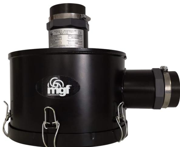
Filtration kit with HEPA H14 element for dental extraction. This kit can be used for all types of dental suction and can be installed either downstream of the exhaust air outlet (wet suction) or upstream (dry suction). It is easy to install and maintain. The kit also includes the fittings necessary to adapt the filter to 30 and 40 mm diameter tubing, both at the filter inlet and outlet.
