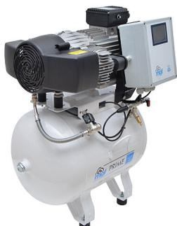
Oil free air compressor IOT version, 2-cylinder, with an air output of 170 l/min at 5 bar pressure. Tank capacity 40 L, internal surface treatment to protect against corrosion.
