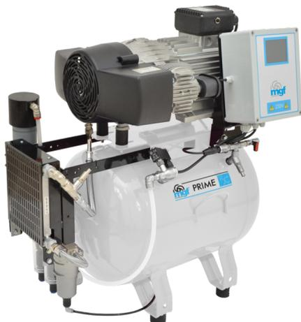
Oil free air compressor IOT version, 2-cylinder, with an air output of 152 l/min at 5 bar pressure. Tank capacity 40 L, internal surface treatment to protect against corrosion.
