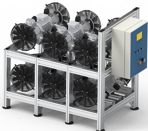
The CENTRALAIR 6 centralized unit is a oil free compressor with a capacity of 2,700 l / min at 5 bar and an adjustable maximum pressure from 8 to 10 bar. The control unit is able to regulate the operation of the pumping elements as to guarantee constant pressure to the system.
